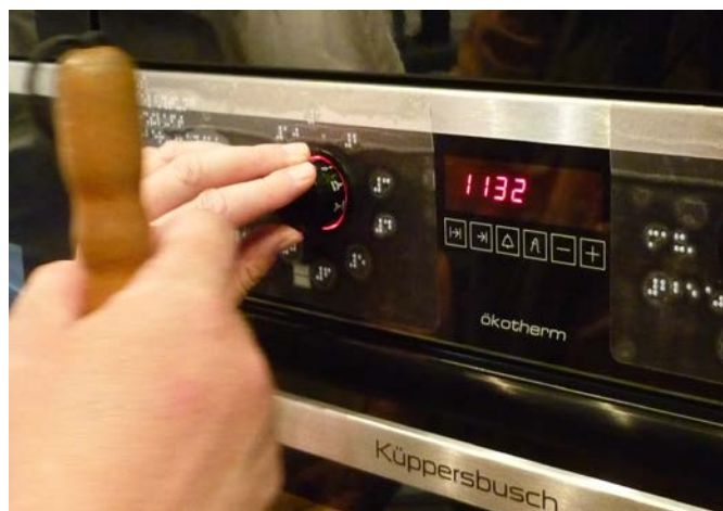
Picture 4: DBSV Küppersbusch / Oven with a braille tape around the rotary selector © DBSV
